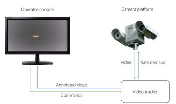
video tracking. The proposed imaging subsystem integrates a hardware-based video tracking system with robust detection and target tracking software for complex image processing applications. The video tracker analyzes video image sequences from the imaging sensor, mounted on a servo controlled pedestal to keep the camera pointing at the nominated object. In this context, the tracker has two primary processing functions:
