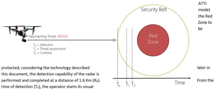
engagement with the target, with the scope of assessing the real threat level and preparing the response, if needed. The presented architecture and the technology allow the accomplishment of the task in less than 15 seconds (therefore  $T_1=T_0+15$  seconds), therefore:
